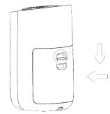
5. Put the filter door back in place – squeeze the button on the door to reinsert.
