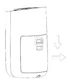
1. Open the filter door by squeezing the button on the door to release.
