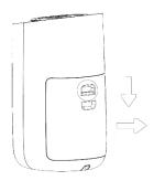
1. Open the filter door by squeezing the button on the door to release.
