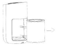
2. Push the filter down and twist it clockwise to remove.
